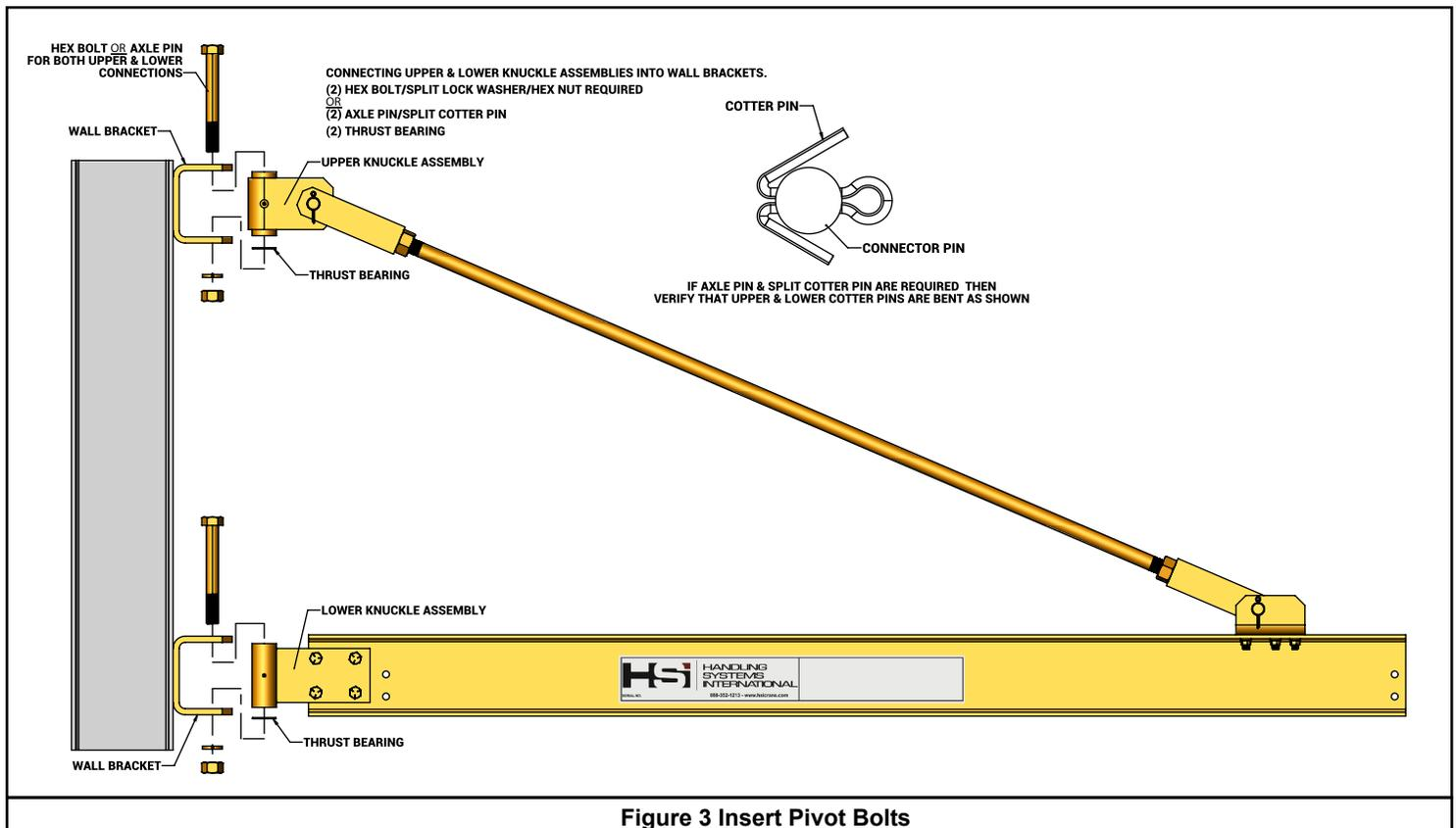
11. Check jib for plumbness by permitting crane to swing freely. Make adjustments by shimming where needed. Elevation of BOOM may be adjusted by loosening or tightening NUTS on the RODS. Make adjustments where needed.
