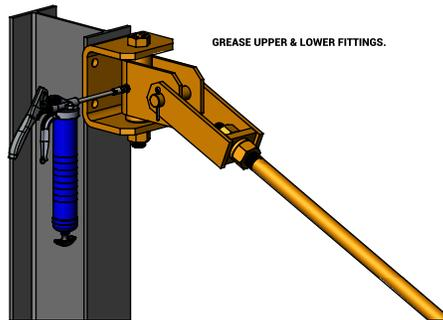
13. Check Rotation of jib for alignment, binds, or slow downs. Make sure all obstructions or interferences are removed.
